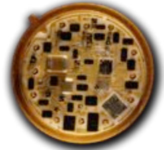
Fig. 1b – Extracted Silicon Die Re-Assembled Into MCM Hermetic Package
