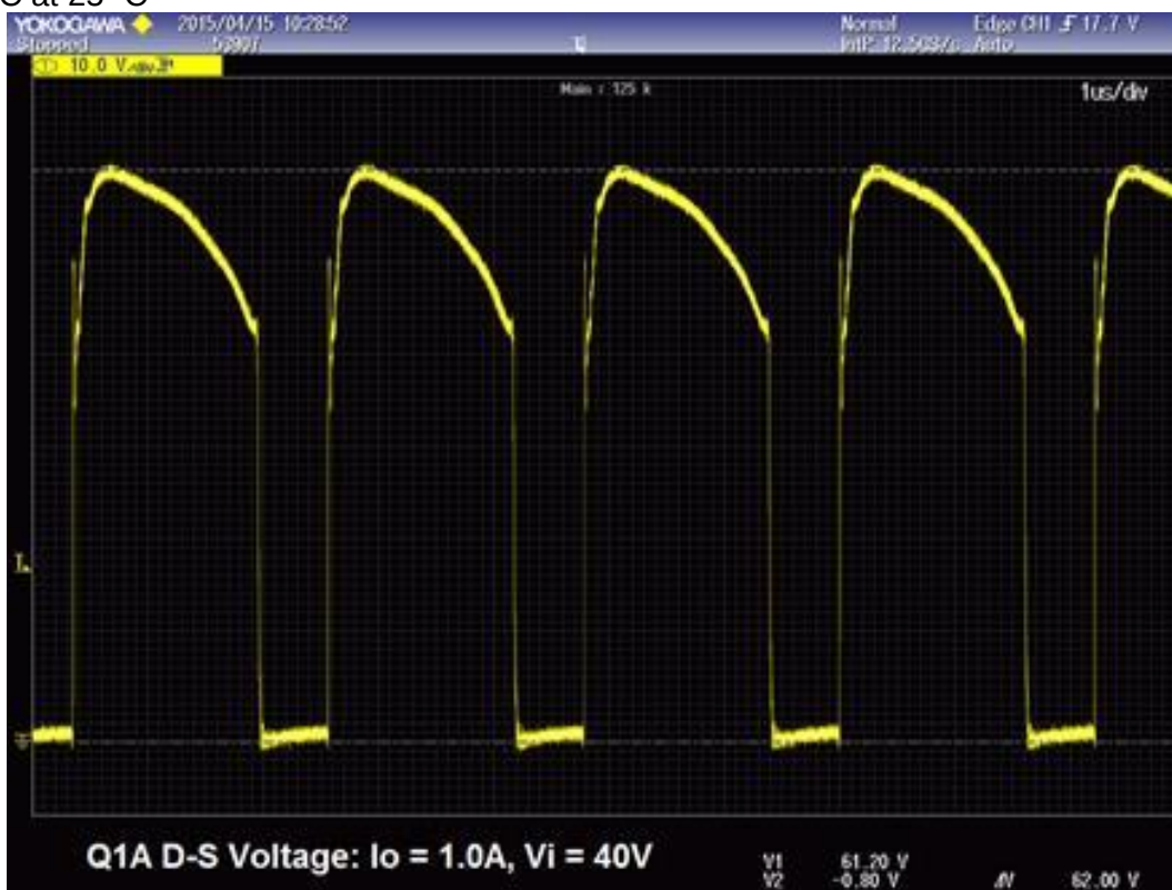
Fig. (13) Healthy Voltage waveform across MOSFET without any high Voltage spikes caused by the leakage inductance at 25 °C
