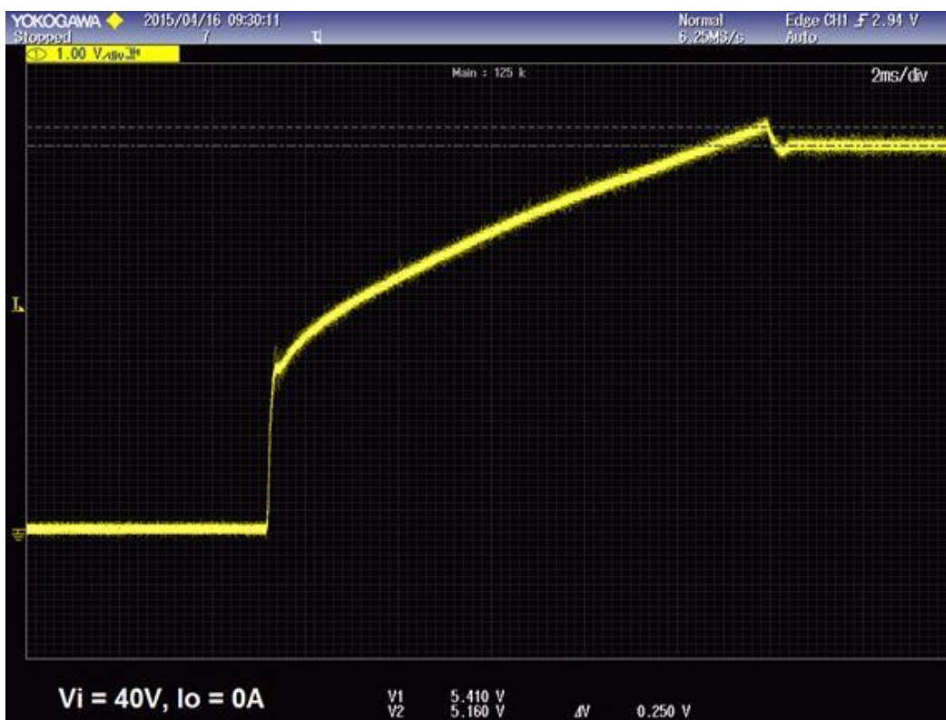
Fig. Fig. (12) Turn ON output voltage transient at no load and maximum line input voltage of 40 VDC at 25 °C
