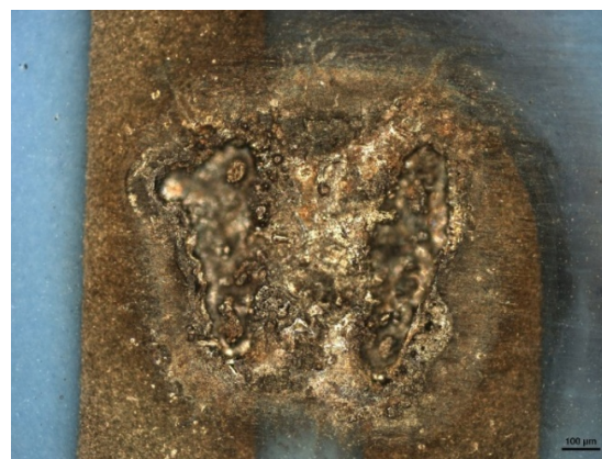
Figure 5. Micrograph of deteriorated DP 9615 glass protective layer after function test
