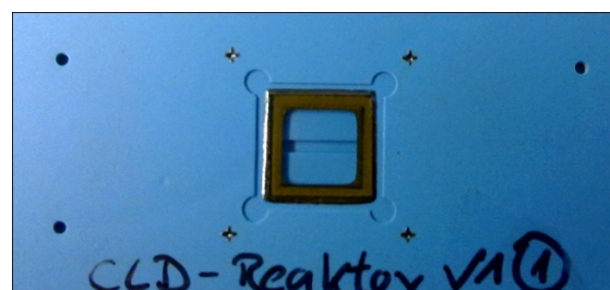
Figure 9. Top view of a CLD chamber with glass window
