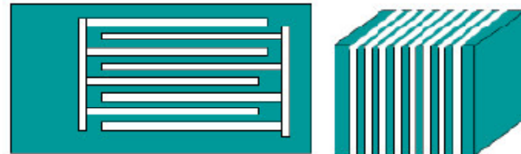
3. Sputter Cu and electroplate Cu to fill the channel
