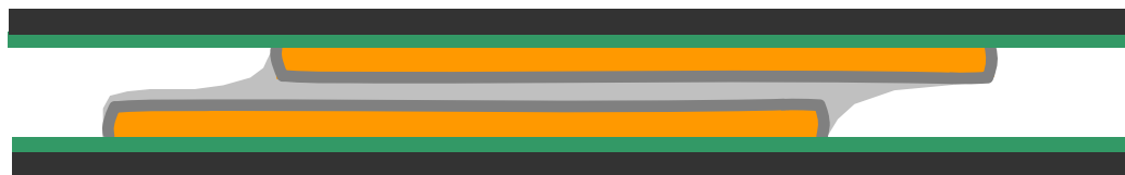
SLID intermetallic formation intermediate phase
