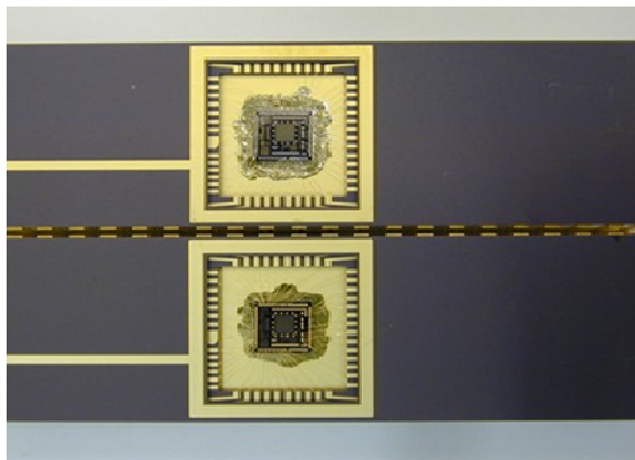
Fig 2. Samples of SOI devices assembled in HTCC package for assessment of electrical performance at 250°C
