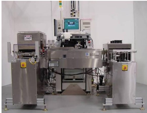
Figure 11 – Through Conveyor System with Odd-Form Part
