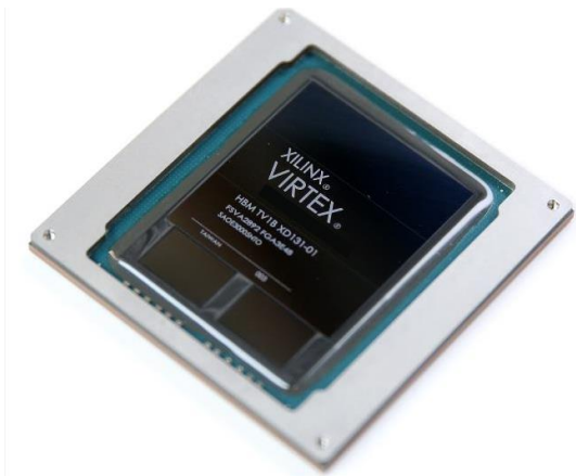
Figure 2: Xilinx Ultrascale+ FPGA-HBM Integration
