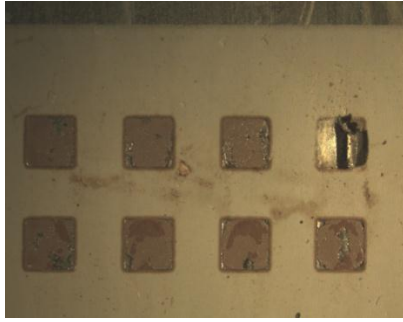
Figure 9: Pad Lift Failure Mechanism.
