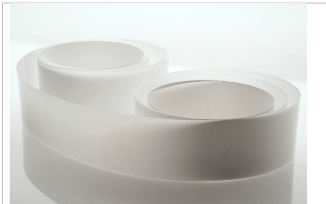
Figure 1 Ultra-thin alumina ceramic has thermal and electrical properties to enable a paradigm shift in power electronics packaging
