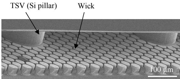
Fig. 3 SEM Si vapor chamber TSV chip (bird's eye view)
