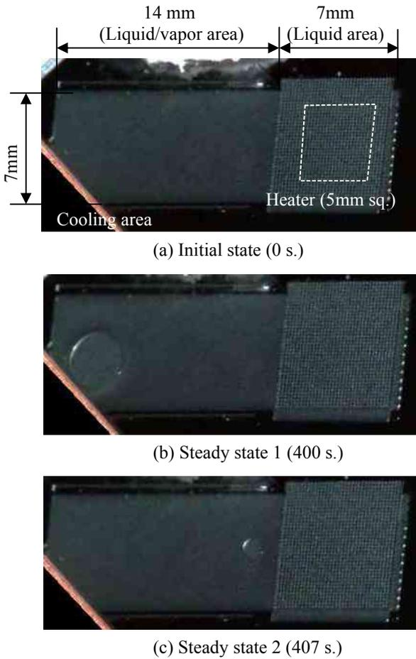
Fig. 9 Liquid behavior in the no-TSV samples
