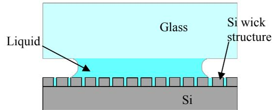
Fig. 8 Appearance of liquid at the center
