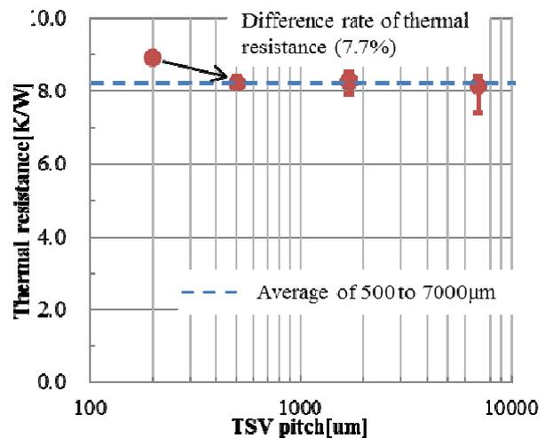
Fig. 11 Relation between Si pillar pitch and the average thermal resistance (all cases have working fluid)
