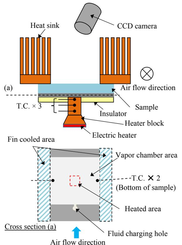
Fig. 6 Schematic of the experimental setup
