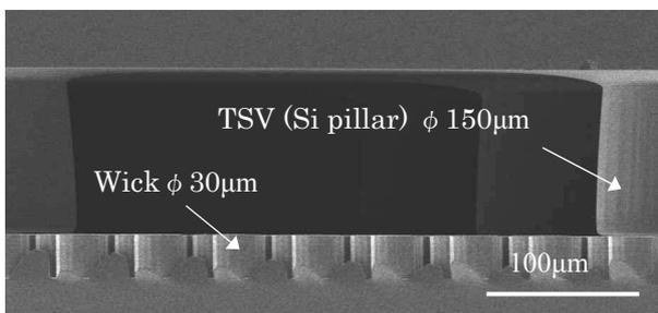
Fig. 4 SEM photograph of wick & TSV structure for Si vapor chamber (cross section)
