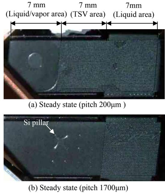
Fig. 10 Liquid behaviors in TSV (Si pillar) samples
