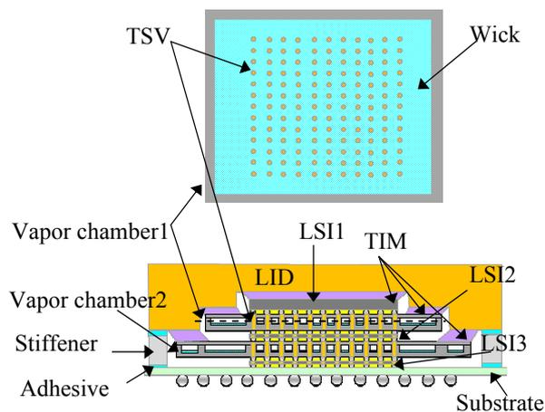
Fig. 1 Structure of a 3D package embedded vapor chamber chip (upper) cross section view of vapor chamber1, (lower) cross section of the package
