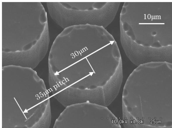
Fig. 5 SEM photograph of wick structure
