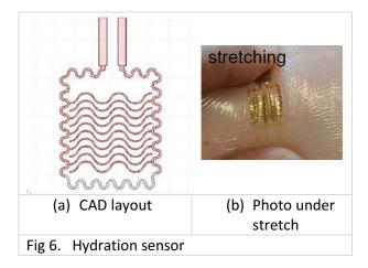
The sensor was designed with aid of detailed FEM calculations, to be reported later. The sensor is shown relaxed and in tension in Fig 7.
