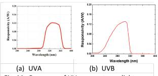
Fig. 11. Response of UV sensors to sunlight.
