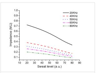
Fig. 8. Impedance of sensor as a function of hydration and measurement frequency.
