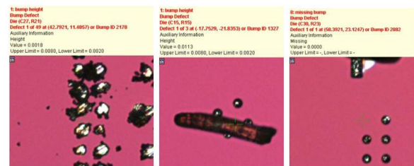
Figure 13 - Detected defects included (left) fragmented, misshapen, poorly formed bumps; (center) contaminating debris; and (right) missing bumps.
