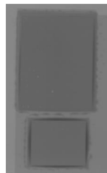
Figure 4. Representative X-Ray image of die attach on thin-film substrates
