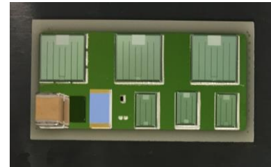
Figure 1. One of the test vehicles assembled on a Ag thin-film substrate
