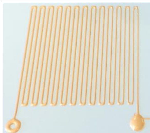
Fig. 2: Robocast Ag ink on unfired LTCC
