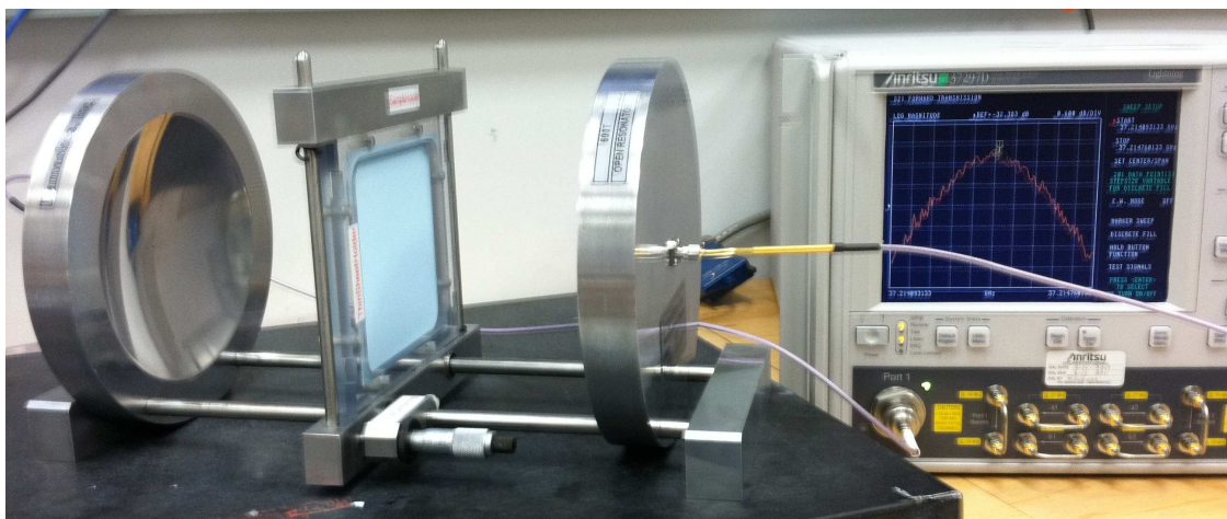
Figure 1: Open resonator test setup with the test sample centered between the concave reflectors.
