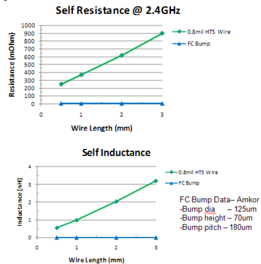
Fig. 1: Electrical Performance of FC vs. WB at 2.4 GHz [16]
