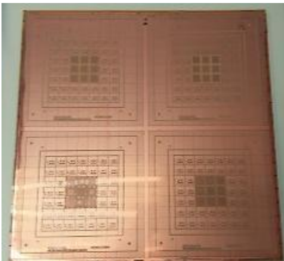
Figure 5: With proper handling and protection methods, no glass cracking seen after Cu plating process
