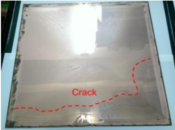
Figure 4: Glass crack occurred in copper plating process
