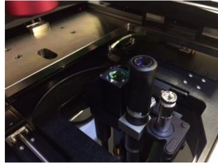
Fig. 2. Internal view of the bottom head optical system for 3D integration combining thickness metrology and IR inspection
