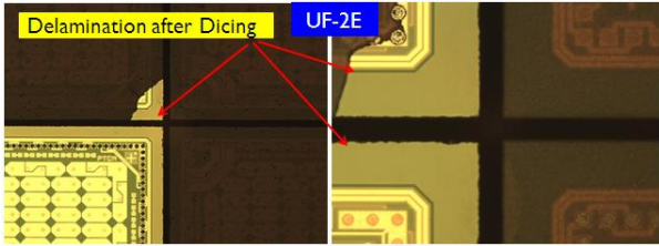
Fig. 15: Delamination observed after dicing the test vehicle with WLUF.
