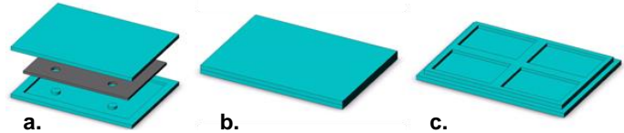
Fig. 3. TPG composites are made by encapsulating TPG in metal cladding. The composites can be machined for specific applications. Steps from left to right are a) cutting TPG and inserting into metal clad; b) bonding; c) post-bonding machining.
