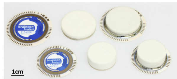
Figure 2: Different substrate, lid and package designs for the Braincon implant. Top row: 36 mm screen-printed alumina substrate, lid (ø=27 mm, height h=5 mm, wall thickness d=1 mm, fillet R_f=1 mm) and fully-assembled package. Bottom row: 30 mm substrate, lid (ø=21 mm, h=8 mm, d=1 mm, R_f=1 mm) and corresponding assembly.
