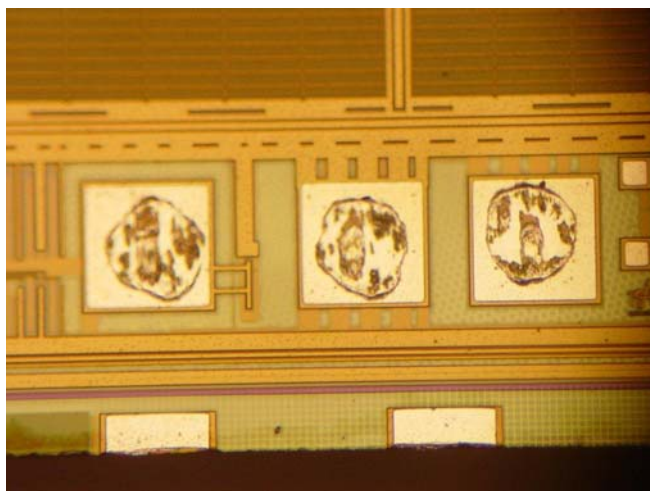
Figure 8. Gold ball removed from aluminum pads. Note the absence of IMC formation under the original pad. Also note the impression remaining after the bump has been removed.
