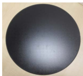
Fig. 8 Molded fan-out wafer
