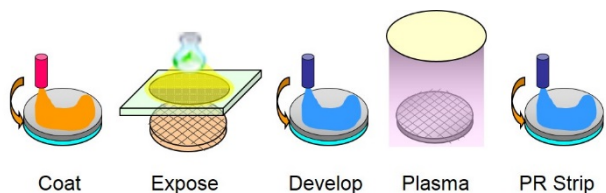
Figure 5. Conventional photolithography based plasma etching process flow.
