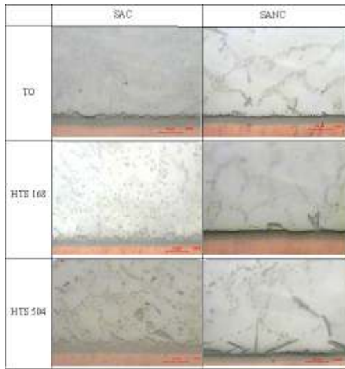
Figure 6. Morphology of intermetallic compounds formed at the interfaces for SAC and SnAgNiCo after high temperature storage
