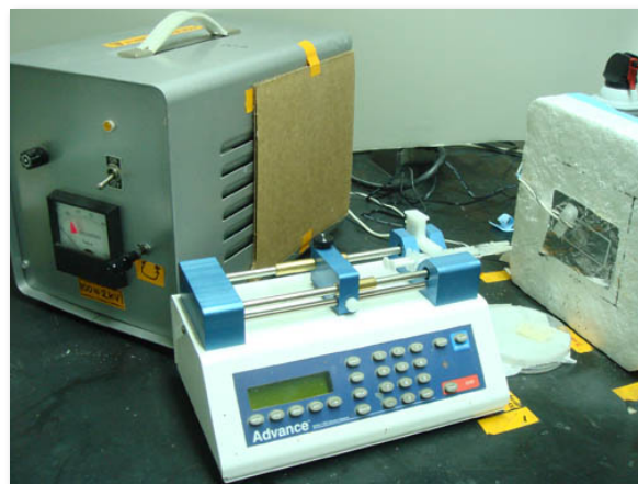
Figure 1: This is the electrospinning set-up used to make titania nanofiber mats; (clockwise from bottom) syringe pump, high voltage power supply (HVPS), conductive collecting substrate.
