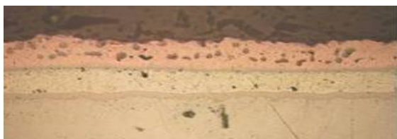
Fig. 11 TEC element solder joint cross section.
