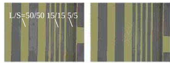
Figure 17: Redistributed layer on planar layer
