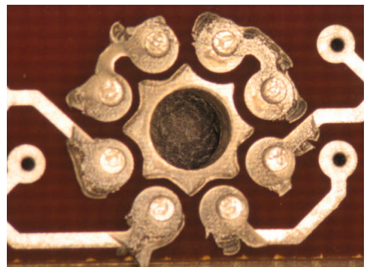
Pads of the board at flex/polyimide level ("button" side)
