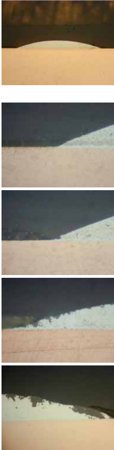
Fig.18 Optical microscope images of corrosion (holding time; 0-1000h) (the upper is 0h ,the second is 30h, the third is 100h, the fourth is 300h, the bottom is 1000h)
