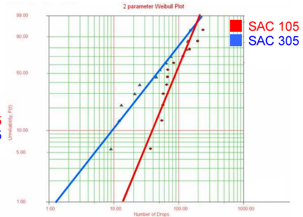
Figure 19: Drop test Weibull plot comparison of SAC 105 v/s SAC305
