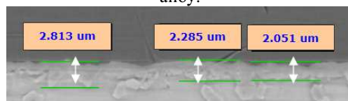
Figure 16: Temperature cycling- (\text{Cu,Ni})_6\text{Sn}_5 Intermetallic at the package side for the SAC 105 alloy.
