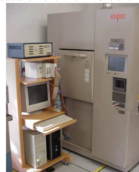
Figure 8: Thermal cycling test chamber and data monitoring system
