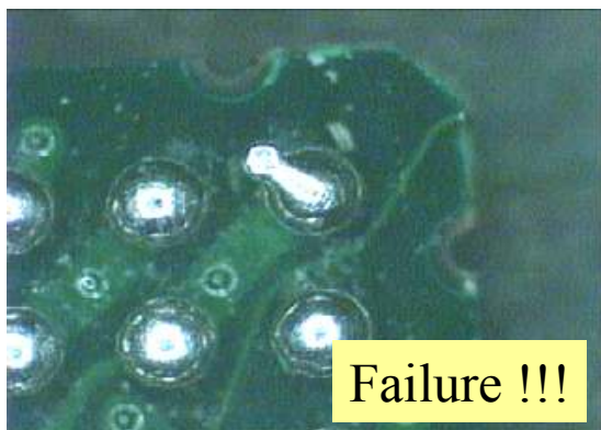
Figure 7. Solderability test failure mode: satellite ball
