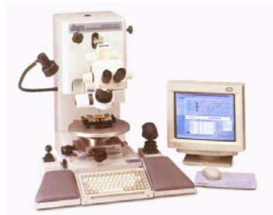
Figure 11: Visual Inspect of Die Sheared Material Using a Microscope
