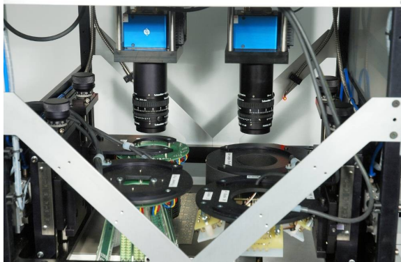
Fig. 15: AOI image head with two cameras
