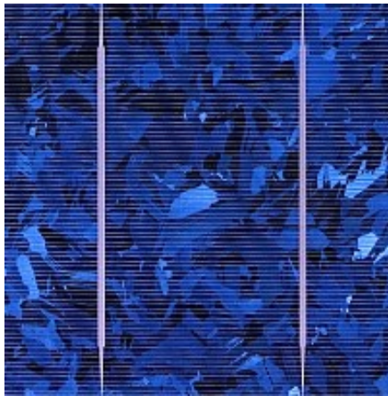
Fig. 7: If polycrystalline silicon is illuminated with direct light the grain boundaries are visible and dependent on the angle of the light the grains are highlighted.
