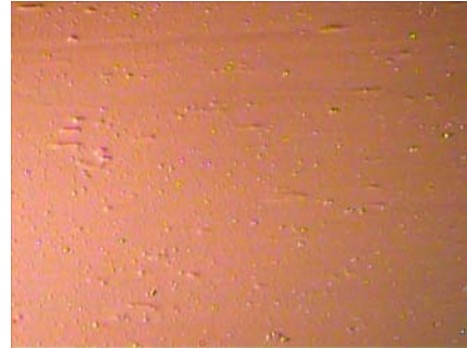
Figure 4. A gold slurry printed on an alumina substrate. The tiny dots are the agglomeration of gold particles.
