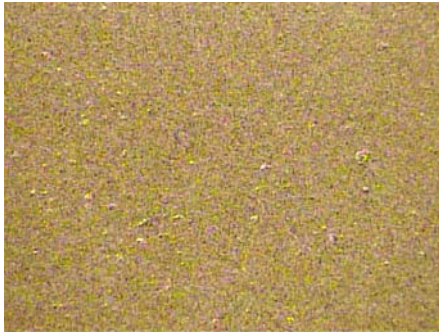
Figure 2. Solid irregular shaped dots on a printed gold surface.
