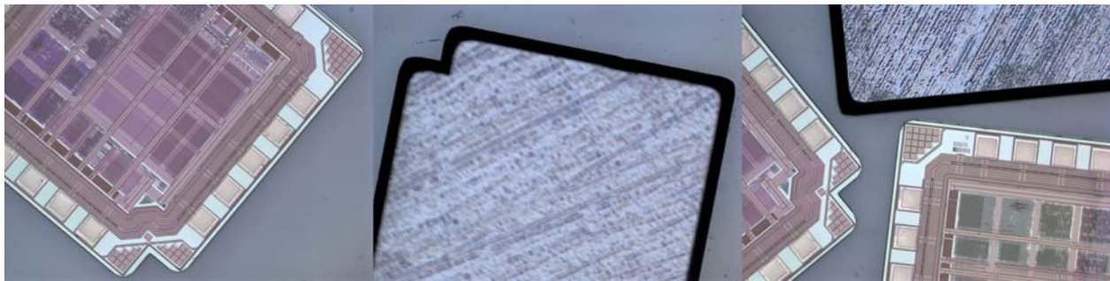
Figure 1. Squared chips include a 250 \mu\text{m} x 250 \mu\text{m} notch to achieve asymmetrical shape. (ASIC– designed and fabricated at CNSE).
