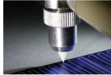
Figure 2 Pen tip printing fine lines on a solar cell.
