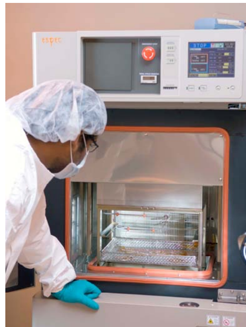
Figure 2: ESPEC Thermal Shock chamber used for accelerated aging of the samples.
