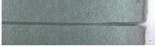
(b) UF-A at 58°C after critical fracture
