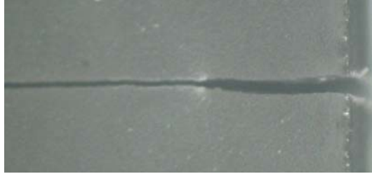
(c) UF-B at -46°C after critical fracture
