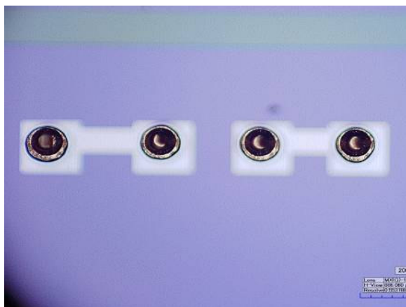
Figure 1: Stud bumps on die bondpads after coining.
