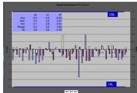
Figure 14: Laser Mark Head Placement Accuracy Results
