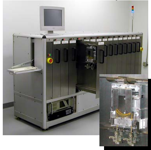
Figure 5: High performance curing system (Inset: Aerospace cable assembly in precision work pallet)
