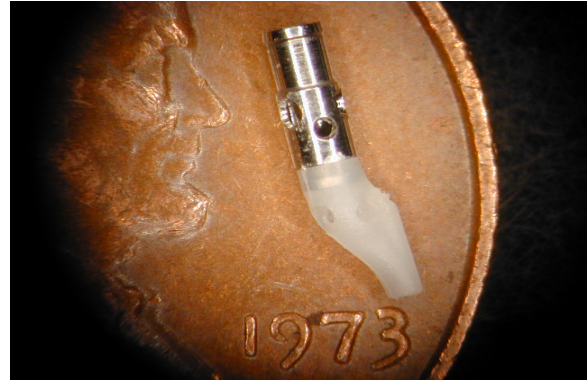
Figure 7: Micro over molding of metal component.
