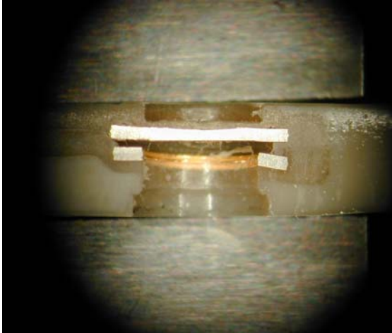
Figure 2: Side view of distorted metal insert in over mold.
