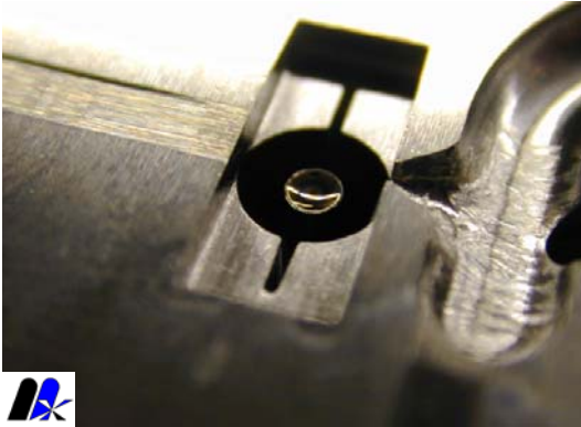
Figure 4: Mold cavity with diamond turned insert.
