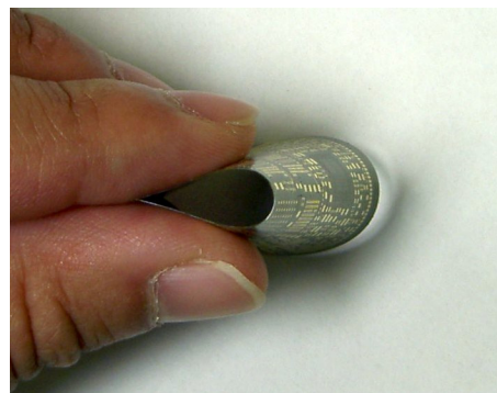
Figure 7. Bending the 7-layer SIP substrate
