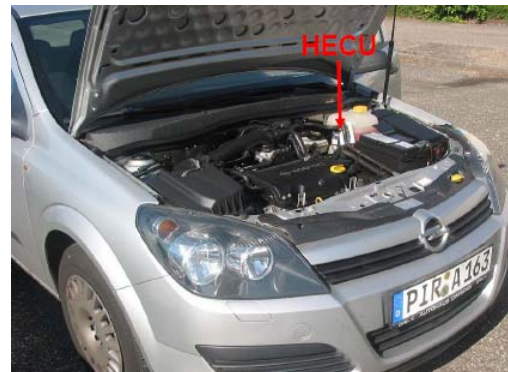
Figure 4 & 5 – Typical location of ESC system HCU
