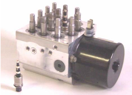
Figure 2 – Typical Hydraulic Control Unit (HCU) for an ESC system
