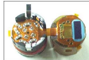
Figure 13 – View of the flipchip and surrounding materials.
