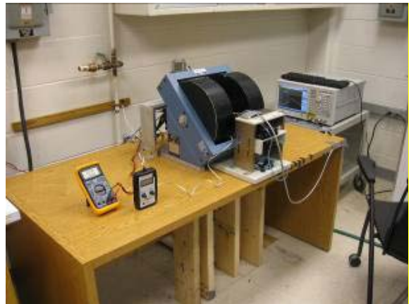
Figure 5: Two-port microwave test setup with well-calibrated external magnetic field applied by the electromagnet
