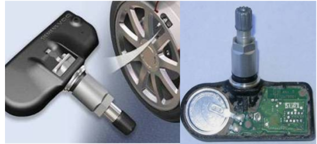
Figure 12: Left, sensor showing wheel mount location. Right, back of sensor with potting compound removed
