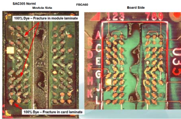
Figure 11 Typical dye-pry for FBGA packages.
