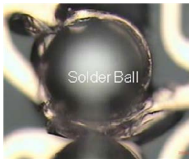
Figure 6 shows the solder ball after ball shear test for solder ball over the die area.
